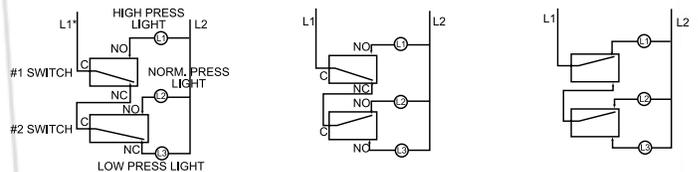
Condition: Pressure level at or below low; Pressure low; Pressure light on, others off
