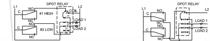
(a) At high pressure relay is energized Load 1 is de-energized Load 2 is energized
