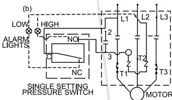
Connect pressure switch same as (a) or (b) for desired motor response to Press. change (a) as shown above
