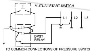
Insert relay as shown in line between LI and common connections of pressure switch. Connect as in Diagram 5 for motor action.
