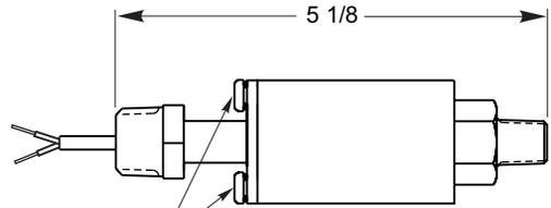
**H5-E 1/2 NPT CONDUIT ELECTRICAL CONNECTION
